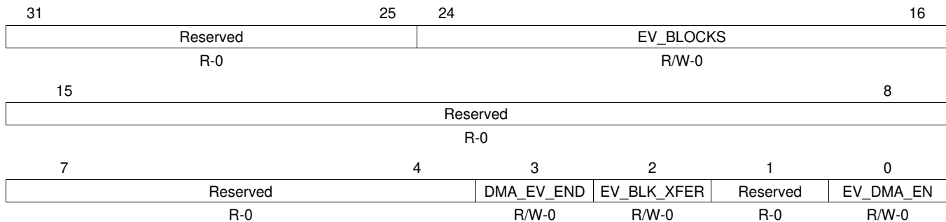
Figure 19-40. ADC Event Group DMA Control Register (ADEVDMACR) [offset = 4Ch]
