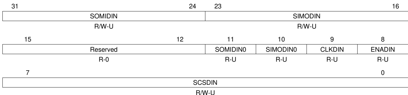
Figure 24-33. SPI Pin Control Register 2 (SPIPC2) [offset = 1Ch]
