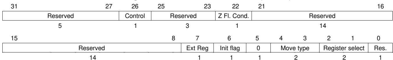
Figure 20-154. MOV32 Control Field (C31:C0)
